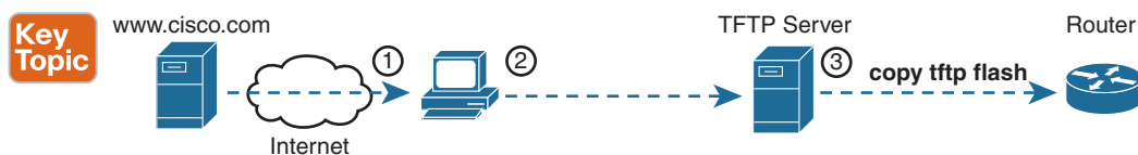
Figure 12-13 Copying an IOS Image as Part of the Cisco IOS Software Upgrade Process
