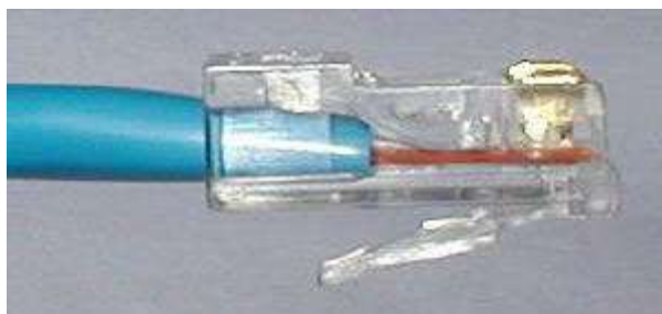
Fig 1.11 Wires in RJ 45 Connector
